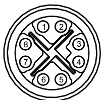
Figure 27: 8-Pin M12 X-Coded Ethernet Port Pin Configuration
