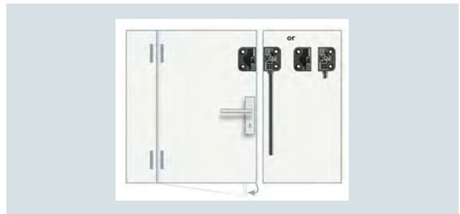
Non-contact safety magnetically operated switches (with plug or cable) for left-hinged door
